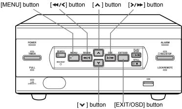
You can check the date/time of power failures and the amount of hard disk operation time.
